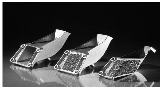
Figure 7 Prototype of a BMW engine mounting bracket manufactured by LKR Ranshofen (Austria). From left to right: empty casting, entire composite part consisting of foam core and cast shell, section through composite part (courtesy of LKR)
