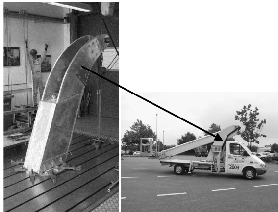
Figure 4 Base of a lifting arm made from AFS sandwich panels. Manufacturer is Advanced Light-weight Materials GmbH in Saarbrücken, Germany (courtesy of ALM)
