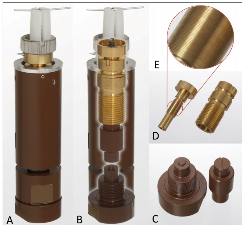
FIG. 2. Compression device used for high resolution tomography of circular GDL samples. (a) Total view; (b) transparent total view revealing interior details of the construction; (c) sample holder basis (left) and compression punch with integrated channel structure mimicking the flow field channel geometry (right); (d) hollow adjustment screw and sleeve made of brass; and (e) detail of the adjustment screw showing the male ultra-fine thread (pitch = 200 \mu\text{m} ).
