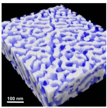
Figure 7: Transmission electron microscope (TEM) tomographic reconstruction of nanoporous gold (Courstesy of M. Chen, Materials Research Tohoku University).
