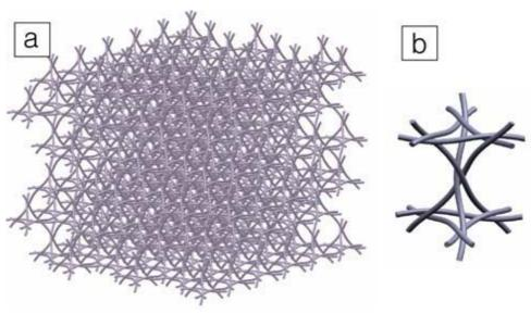
Figure 3. a) Wire-woven Bulk Kagome (WBK) structure and b) unit cell (courtesy of Y.H. Lee, Chonnam National University).
