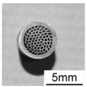
Figure 4. Cross section of tubular structure obtained by extrusion and sacrificial leaching (Courtesy of H. Koh from the Osaka University).
