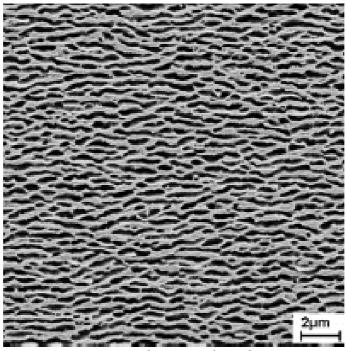
Figure 6. Microstructure of a  $\gamma$ -membrane with submicron aligned porosity obtained after dissolution of the  $\gamma$ -phase in Ni-based superalloys [Fehler! Textmarke nicht definiert.].
