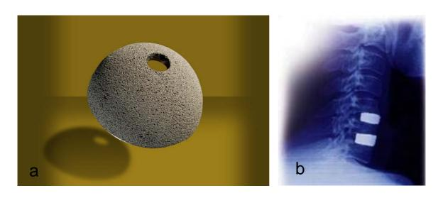
Figure 5. Porous titanium coating on an acetabular cup for hip replacement (Courtesy of National Research Council Canada, Industrial Materials Institute) and b) porous Nitinol for cervical vertebra fusion (Courtesy of Biorthex).
