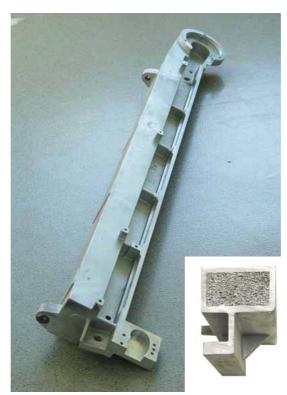
Figure 9. Girder (a) cross section showing Alporas foam core, (b) entire part, length = 1900 mm; foam core 1580 mm (Courtesy of Sönke Reinhardt).
