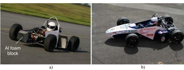
Figure 10. Crash protector in a model racing car built by students at the University of Technology of Stralsund, Germany; a) view of car with the front encasement taken off, b) full view (Courtesy of Sönke Reinhardt).
