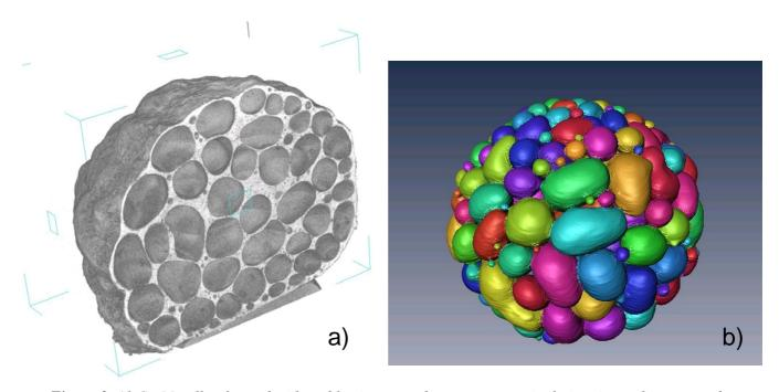
Figure 2. Al-Cu-Mg alloy foamed without blowing agent by pressure manipulation, i.e. melting a powder compact under 6 bar pressure (Argon) and releasing pressure to 1 bar; a) visualisation of foam by X-ray tomography, b) computer-assisted segmentation of individual pores in the sample (courtesy of F. García-Moreno, HMI Berlin).
