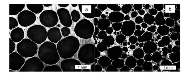
Figure 3: Pore structure of (a) AlMg15Cu10 and (b) ZnAl3.3Mg3.3 foam
