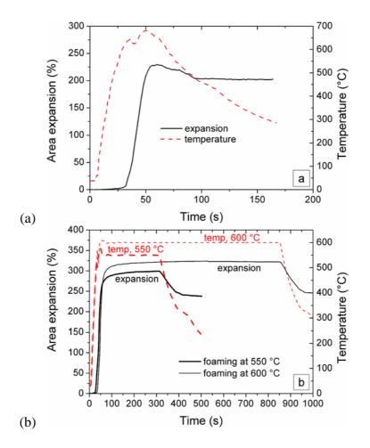
Figure 2: Expansion behaviour of (a) AlMg15Cu10 and (b) ZnAl3.3Mg3.3 alloys
