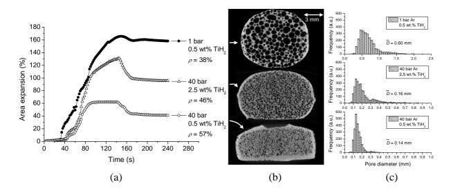
Figure 5: (a) Area expansion during foaming, (b) pore structure and (c) 3D pore size distribution of AlSi6Cu4 foams foamed with 1 and 2.5 wt.% TiH<sub>2</sub> under 1 or 40 bar argon pressure.
