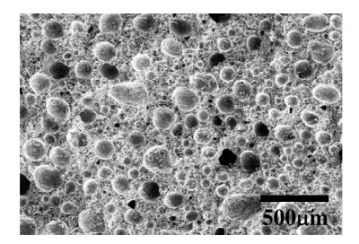
Figure 7. SEM micrograph of a ZnAlMg foam with a relative density  $\approx 60$  %.
