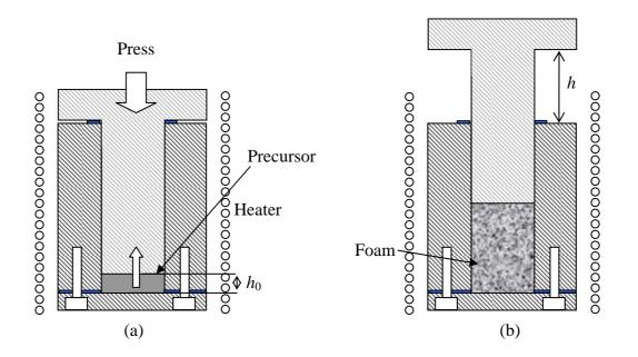
Figure 6. Simplified sketch of two stages of the foaming process, (a) before and (b) after foam expansion.
