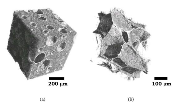
Figure 8. 3D rendering of synchrotron X-ray microtomographies of ZnAlMg foams: (a)  $\approx 60$  % density (b)  $\approx 20$  % density.
