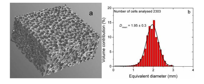
Figure 4: (a) 3D visualisation of X-ray tomographic reconstruction of AlMg15Cu10 foam, Dimension: 20×20×10 mm<sup>3</sup>. (b) Corresponding 3D pore size distribution fitted with a Gaussian distribution curve (reported in Ref. 18).
