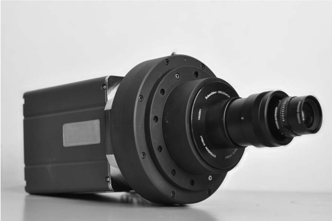
Figure 3: 16-MegaPixel-CCD Camera (Peregrin 486) equipped with a lens of the type Schneider Kreuznach Macro Symmar 5.6/120.
