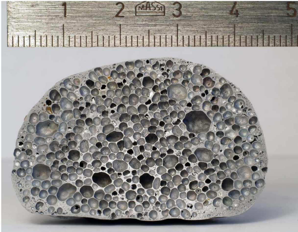
Figure 13: Photographic image of a foam made from AlMg 4 Si 8 alloy, showing a uniform pore structure.
