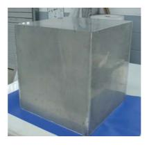
Figure 5. Damping box for electromagnetic waves made of aluminium foam sandwich (AFS). Size is  $1200 \times 600 \times 600$  mm<sup>3</sup>.
