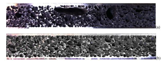
Figure 3. (a) AFS made without carefully adjusting the powder and processing parameters and exhibiting individual large pores. (b) AFS made by applying the current knowledge concerning especially powder degassing. Both AFS: 33 mm foam core and 1.8 mm face sheet thickness
