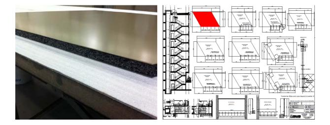
Figure 9. (a) AFS panel used for the base of a stair rail prior to assembly. (b) Drawing of a staircase in a residential building in Geneva containing AFS-supported stair rails. One such element is highlighted in red. In total, 130 AFS segments, each 2.6 m<sup>2</sup> large, were used.
