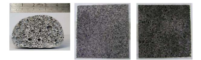
Figure 2. (a) Example of an AlSi8Mg4 foam. (b,c): Two foam samples prepared by cutting an AFS apart along the centre plane. Foams were exposed to salt spraying for 24 h (neutral salt spraying Test according to EN 9227 /ASTM B117). (b) AlSi8Mg4 foam, (c) AlSi6Cu6 foam.
