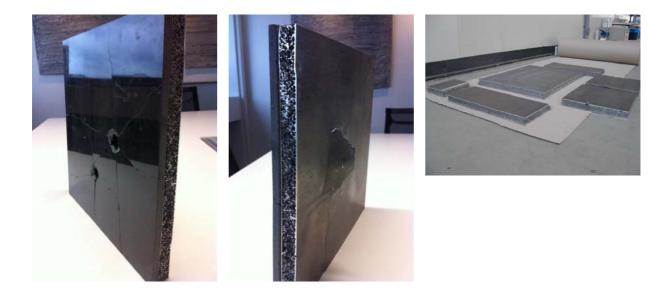
Figure 10. (a,b) Composite of an AFS panel with a polished granite front plate hit by a bullet. The AFS had 1.8 mm face sheets and a 20 mm foam core, while the granite plate was 8 mm thick. (c) Protection for high-speed turning machine built for Kurt Staiger Werkzeugmaschinen GmbH (AFS plates before assembly are shown, size of assembled box is 900×555×755 mm<sup>3</sup>).
