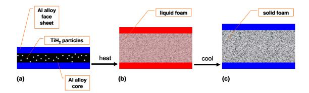
Figure 1. Principle of AFS manufacture. (a) Three-layer composite with a central core layer made of a compacted mixture of metal powders and blowing agent powder, mostly thermally modified TiH<sub>2</sub>. (b) composite expanded upon heating. Only the core is changing its volume, whereas the face sheets remain unchanged.
