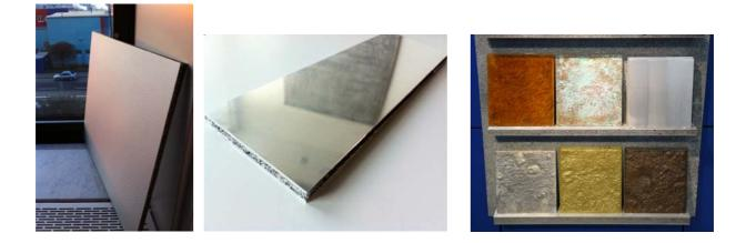
Figure 8. (a,b) AFS architectural plates with (a) dull anodized [18] and structured and (b) shiny polished surfaces, (c) AFS with cor-ten steel, copper oxidized, natural polished, natural amorphous, brass, bronze appearing surface manufactured by coating with a mixture of metal powders and epoxy resin.
