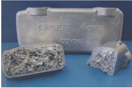
Figure 6. Aluminium foam part made by the 'Combal' process. [366]
