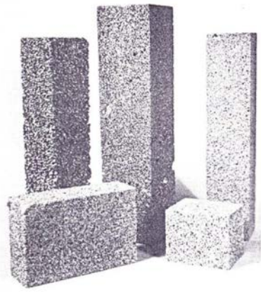
Figure 3. Aluminium foam blocks produced in the 1970s by the Ethyl Corp. [22]
