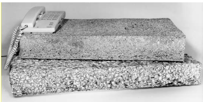
Figure 9. Foam samples made by Hydro Aluminium by blowing gas into SiC containing Al MMCs (Source: Fraunhofer).
