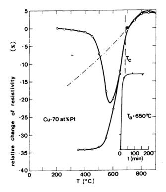
FIGURE 2. Isochronal annealing of Cu-70at%Pt. o rising ♥falling temperature; ■ starting value. Insert: isothermal annealing at 650°C. Dash-dotted: hypothetical SRO-equilibrium line.
