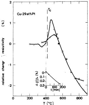
FIGURE 4. Isochronal annealing of Cu-29at%Pt. small decrease of resistivio rising  $\nabla$  falling temperature; starting ty at the beginning of isovalue. Insert: isothermal annealing at 650 °C. chronal annealing (350 °C)
