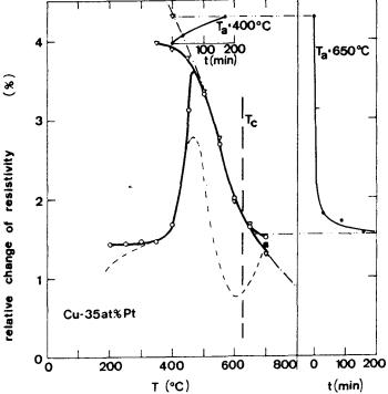
FIGURE 3. Isochronal annealing of Cu-35at%Pt. o rising 💙 falling temperature; 📕 starting value. Inserts: isothermal annealing at 400°C and 650°C. Dashed line: previous run.
