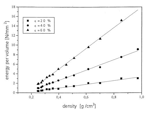
Fig. 4: Energy per unit volume absorbed by various AlSi12 foams after compression strains  $\varepsilon$  of 20 %, 40 % and 60 %.
