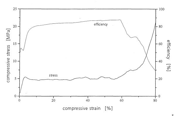
Fig. 3: Compression stress and energy absorption efficiency of an AlSi12 foam ( $\rho=0.36 \text{ g/cm}^3$ )
