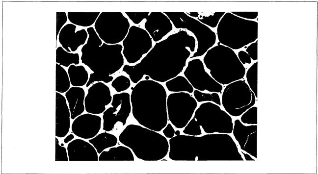
Fig. 1: Cell structure of an aluminium foam (9:1)
