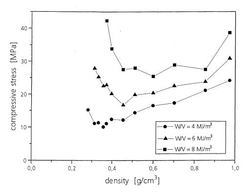
Fig. 6: Maximum stress occurring when a given deformation energy is absorbed by foams of various densities.
