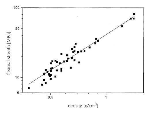
Fig. 2: Flexural strength of AlMg3 foams.
