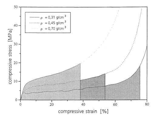
Fig. 5: Compression behaviour of three AlSi12 foams of various densities. The various shaded areas correspond to same absorbed amount of energy W\*.
