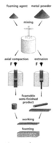
Figure 1: Schematics of processing steps for metal foaming by powder metallurgy.
