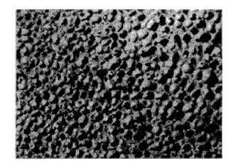
Figure 2: Typical structure of aluminum metal foam produced with powder metallurgy.
