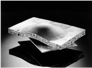
Fig. 9: Composite structure made of an aluminium foam core and steel face sheets (size 250 x 250 x 10 mm<sup>3</sup>)
