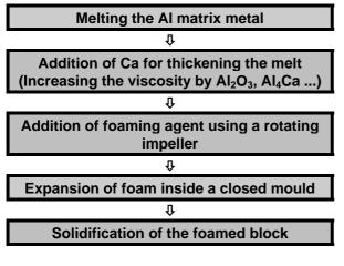
Fig. 2: Direct foaming of melts (ALPORAS-Process)
