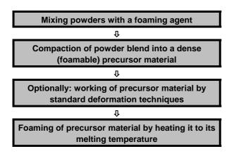
Fig. 7: Powder metallurgical process for making foamed metals
