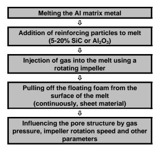
Fig. 1: Direct foaming of melts (MMC foams)
