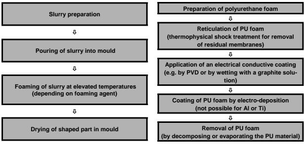
Fig. 14: Foaming of slurries
