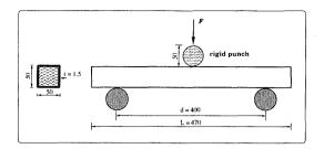
Figure 2: Three point bending test geometry
