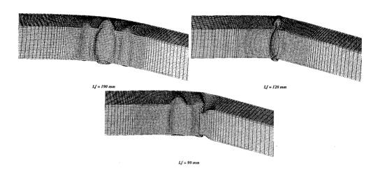
Figure 8: Deformation pattern of partial foam filling
