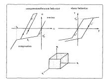
Figure 3: Material modeling of aluminum foam
