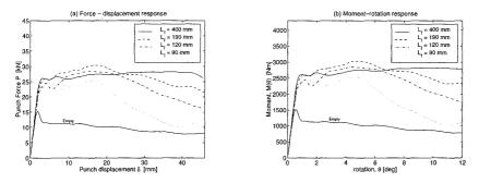
Figure 7: Three point bending response of partial foam filling
