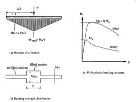
Figure 9: Bending strength and moment distribution of partially foam filled beam
