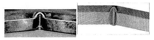
Figure 4: Deformation pattern of empty thin-walled beam
