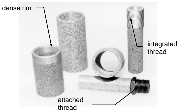
Figure 8: silencers made of aluminium sponge (all except the lying sample are closed on one side)
