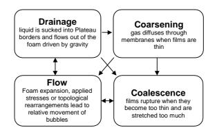
Figure 4: Interdependence of four principal mechanisms in foams.
