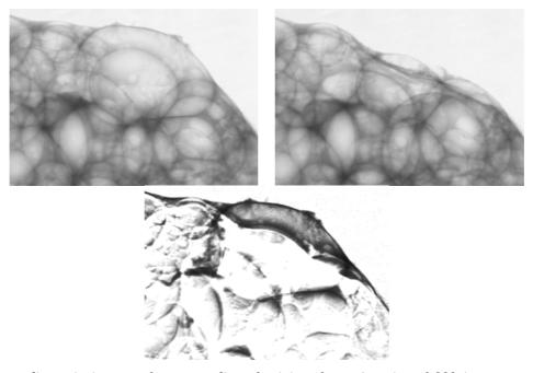
Figure 2:X-ray radioscopic images of an expanding aluminium foam. A series of 900 images was taken with a frequency of 2 per second. Two adjacent pictures and the difference of the pictures is shown. One can see the rupture of an individual cell wall (from [11], see also [12]).
