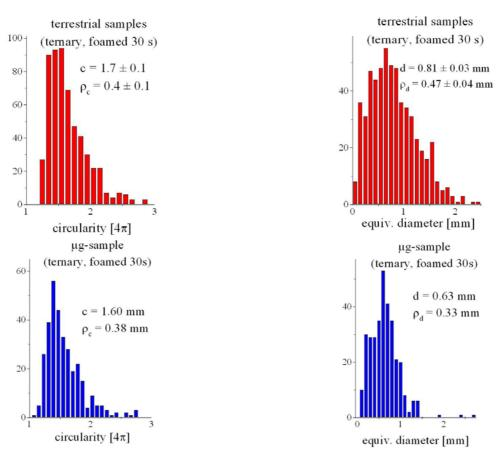
*Figure 5: analysis of lead foams manufactured under 1g (upper panel) and "0g" (lower panel). Circularity (left) and equivalent pore diameter distributions are shown [16].*
