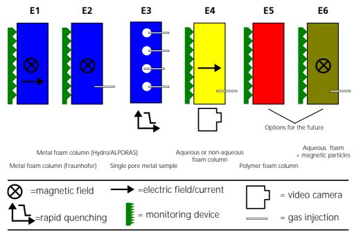
Figure 6: Schematic description of the six planned experiments.
