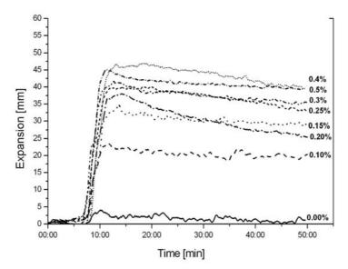
Figure 1: Time dependence of the expansion of AlSi7 alloys with varying content of blowing agent (from [11]).
