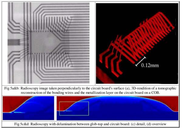
In conclusion we have demonstrated the potential of high-resolution and phase-contrast radioscopy for non-destructive testing of light materials and devices.
