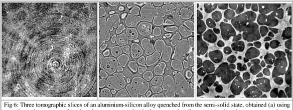
Fig 6: Three tomographic slices of an aluminium-silicon alloy quenched from the semi-solid state, obtained (a) using absorption contrast, (b) using phase contrast and a single propagation distance, (c) using phase contrast and holographic reconstruction based on four distances [4].
