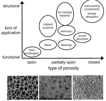
**Figure 7.2-1.** Applications of cellular metals grouped according to the degree of open porosity needed and whether the application is functional or structural.
