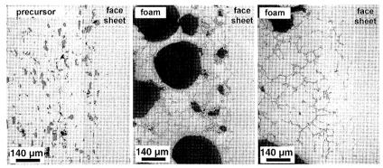
Figure 3.4-3. Metallographic images of sandwich structures with an AlSi7 core. Three different expansion stages are shown: left) unfoamed precursor material; middle) sandwich
