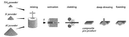
Figure 3.4-1. Process steps for making sandwich panels with aluminum foam cores.
