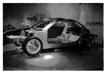
Figure 3.4-4. "Detroit Show Car 1998" developed by Karmann (Osnabrück) for demonstrating potential uses of aluminum foam sandwich panels. The rear bulkhead and the front firewall (not directly visible) are made of AFS.
