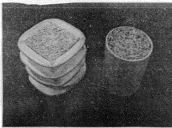
Fig. 2(a) : Prototypes of crash absorbers based on Al extrusions with a filling of Cymat aluminium foam. 2(b) Crash energy absorber for a tram built for the COMBINO vehicle system.
