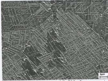
Fig. 9: The microstructure of Re706 after overageing treatment ( 18 \times 10^6 s / 1023K), taken at the SEM.
