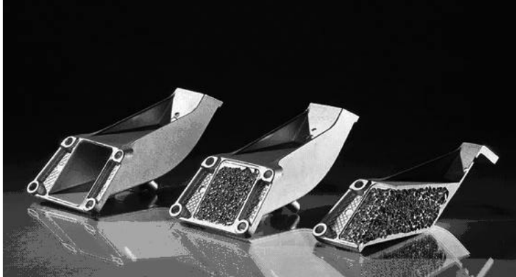
Fig. 5 Prototype of a BMW engine mounting bracket manufactured by LKR Ranshofen. From left: empty casting, composite part consisting of foam core and cast shell, and section through composite part.
