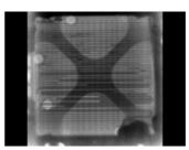
Fig. 2: Radiographic image of a fuel cell. The black horizontal lines are due to the high attenuation of liquid water indicating filled flow field channels.
