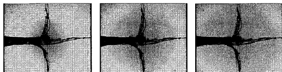
Fig. 2 Imbibition experiments in parabolic flights: picture of a foam at three different times, evidencing isotropic propagation of liquid injected at the center. The wires are connections to electrodes. Note that the wetter foam appears dark. CNES parabolic flight campaign, March 2005 (from ref. 6).
