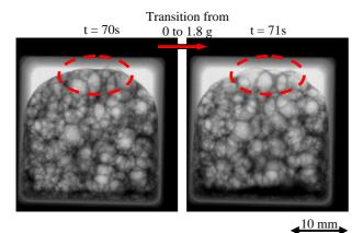
Figure 3. Liquid flow from top to bottom during transition from 0 to 1.8 g in a Thixo AlSi6Cu4 foam. Red ellipses denote the region of interest.
