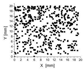
Figure 6. Cell wall rupture map of the Thixo AlSi6Cu4 foam in the liquid state during almost 4 minutes under gravity (left) and during MASER 11 (right) extracted from the sequence of X-ray images.
