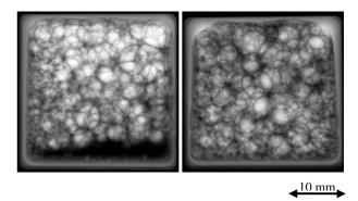
Figure 5. Thixo AlSi6Cu4 sample after 200 s in the liquid state foamed on Earth (left) and during the MASER 11 flight (right).
