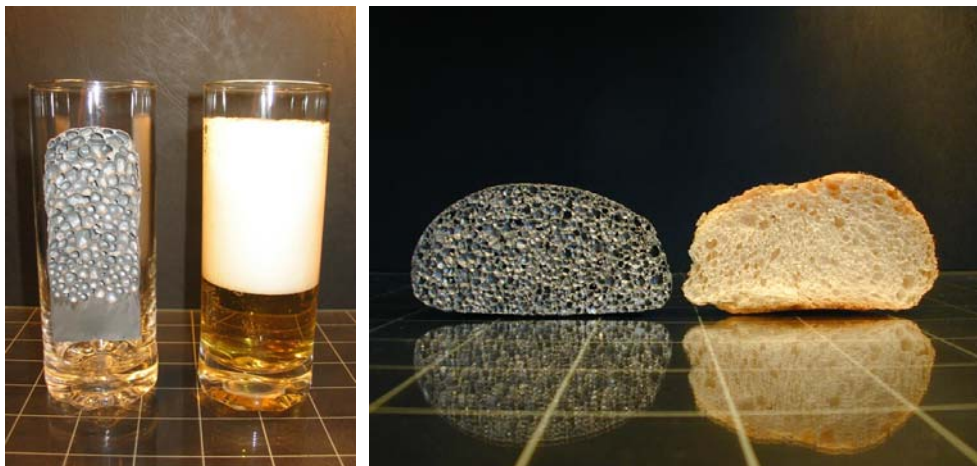
Figure 1. left : aluminium foam blown with air from a particle-stabilised melt and beer, right : zinc foam and bread roll, both foamed by internal gas creation (Photographs: HMI)
