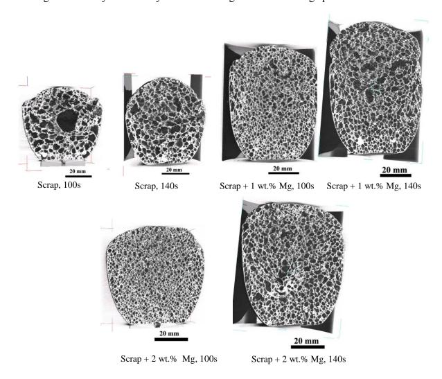
Figure 3. Remelted scrap foam structures (from CT) as a function of Mg content and foaming time at 700°C
