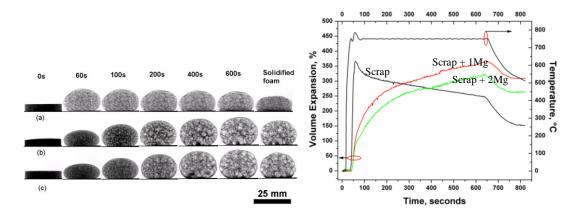
**Figure 4.** Insitu 2D radioscopy of "Formgrip" precursors a) re-melted scrap, b) scrap + 1 wt.% and c) scrap + 2 wt.% Mg (left) and corresponding expansion-time plots (right).
