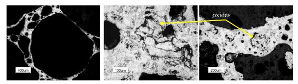
Figure 5. Optical micrographs of cell wall structures for foams made from re-melted scrap
