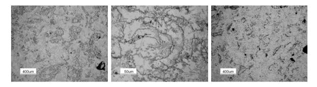
**Figure 2.** Optical micrographs of oxide films and clusters in re-melted scrap alloys (left and centre) and with 2wt.% Mg addition (right).
