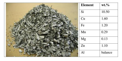
Figure 1. Photograph of the swarf chips and chemical composition (measured by OES)
