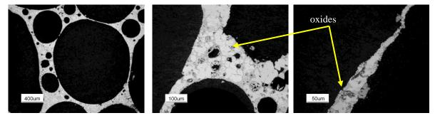
Figure 6. Optical micrographs of cell wall structures for foams made from scrap containing 2 wt.% Mg.
