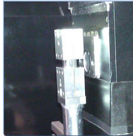
Fig. 2 The investigated PEM fuel cell optimized for high resolution tomography in front of the high resolution detection system. The round-shaped scintillator can be seen in the center of the image.
