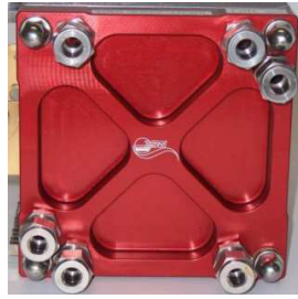
Fig. 1. The investigated PEM fuel cell of the ZSW Ulm. The size was about 140x140 mm.
